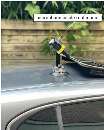
Figure 4. Example of an Anabat SD2 external microphone mounted to a vehicle and oriented at a 45-degree angle. Note that the microphone is directed towards the back of the vehicle to minimize the amount of wind picked up due to the vehicle's movement. Image courtesy of Han Li with the Department of Biology at the University of North Carolina at Greensboro.
