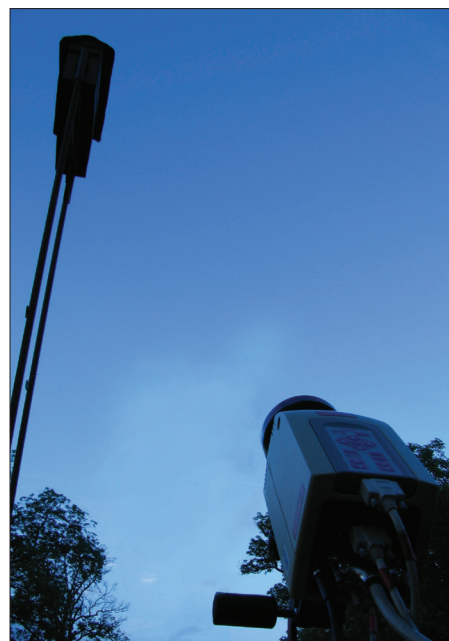
Figure 7.1—Double-observer setup for pairing manual exit count at a bat house with infrared thermal recording of the same emergence activity. (photo by Jonathan Reichard)
